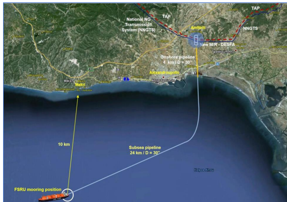
FSRU Location Alexandroupolis.
