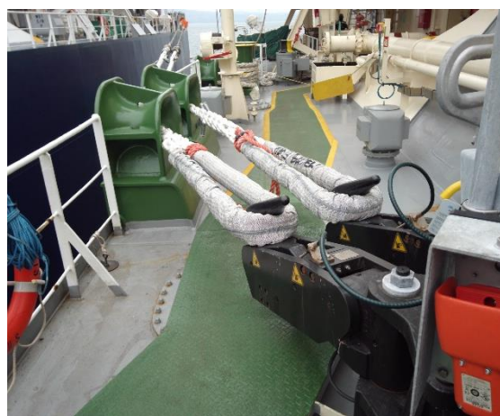
Figure 27 FSRU ALEXANDROUPOLIS - Mooring Hooks
