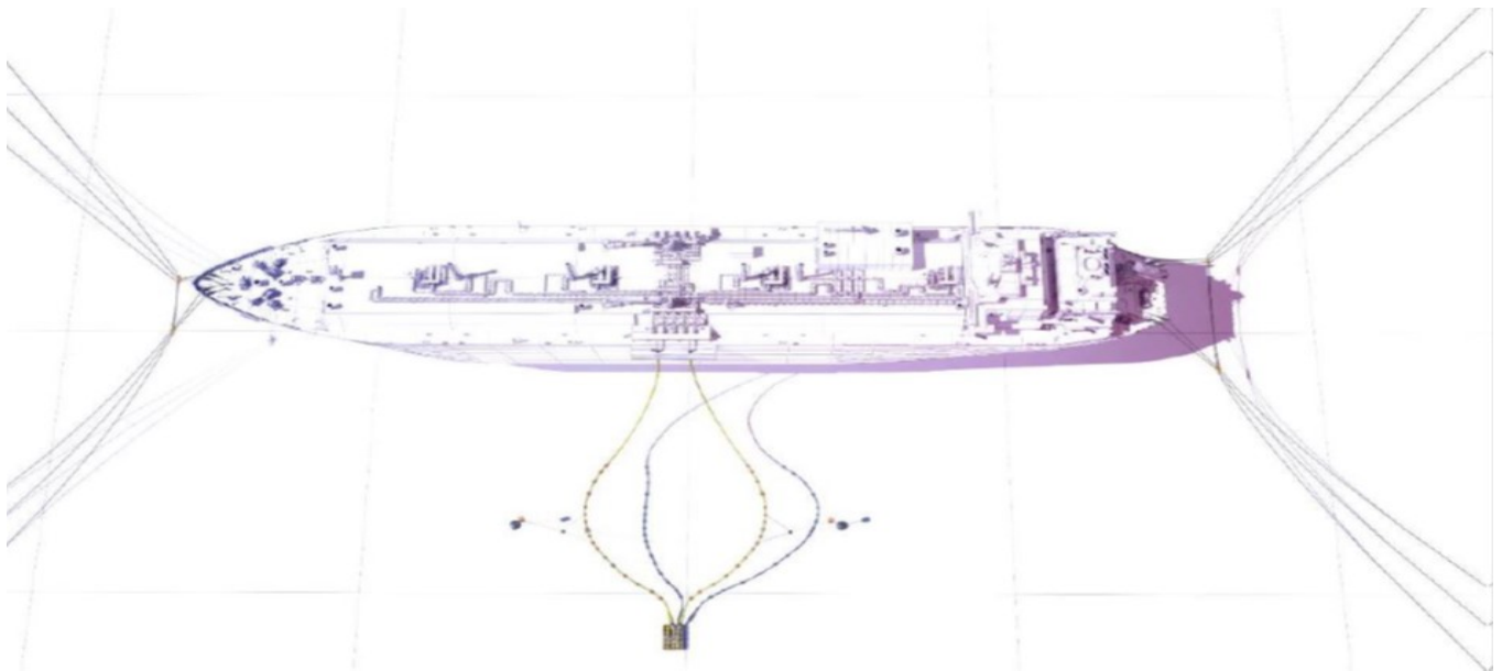
Figure 2.2 – FSRU Restricted Catenary Mooring-RCM
