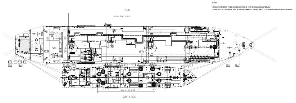
Figure 19 Proposed mooring plan with up to 20000 LNGC
