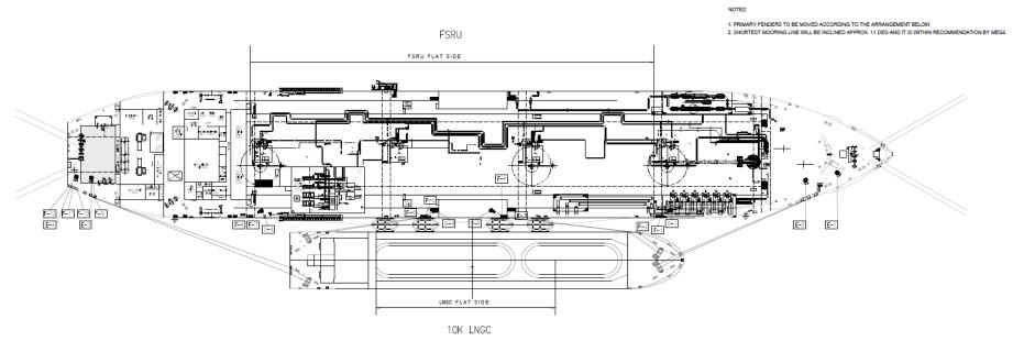
Figure 18 Proposed mooring plan with up to 10000 LNGC
