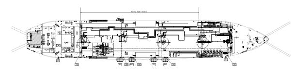
Figure 23 Primary fender position for receiving small LNGC carriers (3K-20K)
