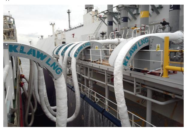
Figure 10 Flexible Hoses during Cargo Operation
