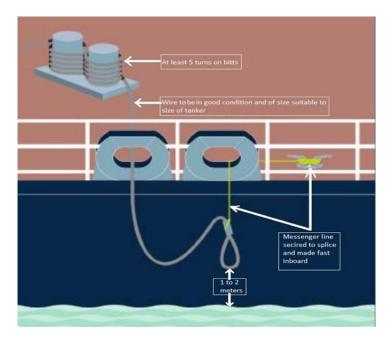
Figure 30 Fire Wire Messenger Line
