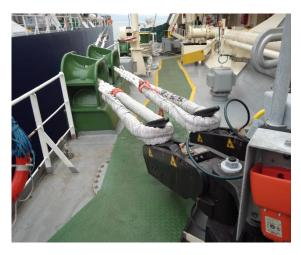
Figure 27 FSRU ALEXANDROUPOLIS - Mooring Hooks
