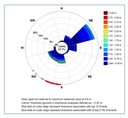
Figure 7 Wave Rose for the FSRU
