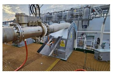
Figure 17 Fall Arrest system on the FSRU
