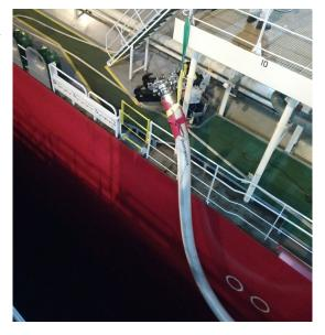
Figure 13 Hose Lifting with hose buns
