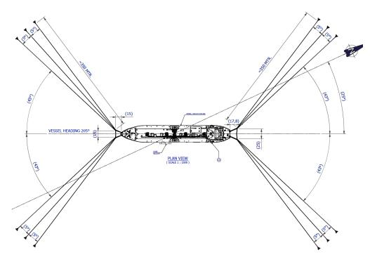
Figure 4 Anchoring Plan - Plan View
