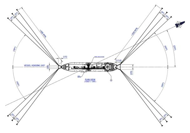
Figure 3 Anchoring Plan - Plan View
