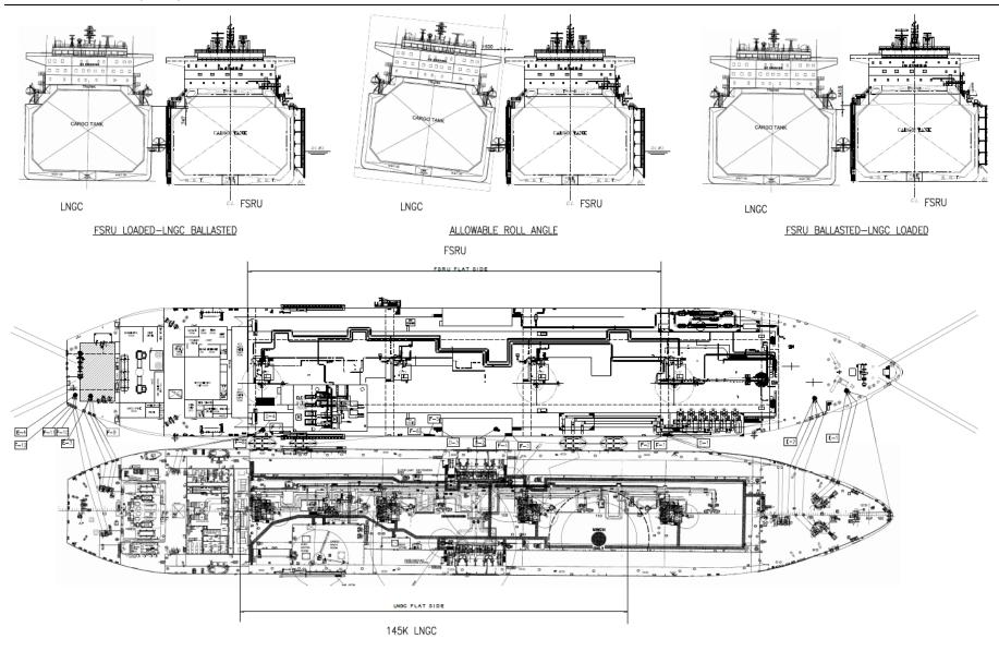
Figure 20 Proposed mooring plan with up to 145000 LNGC
