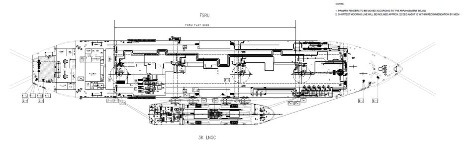
Figure 16 Proposed mooring plan with up to 3000 LNGC
