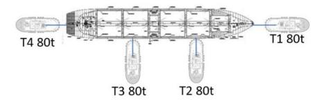
Figure 19 Typical Tug Arrangement
