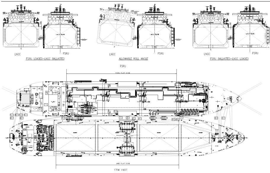
Figure 21 Proposed mooring plan with up to 170000 LNGC
