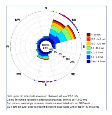
Figure 6 Wind Rose at 10m for the FSRU
