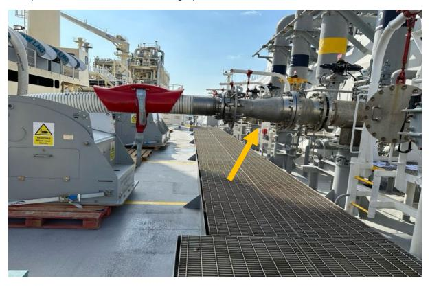
Figure 31 Manifold Reducer
