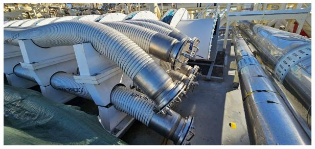
Figure 9 Gutteling Multi-LNG White Hose
