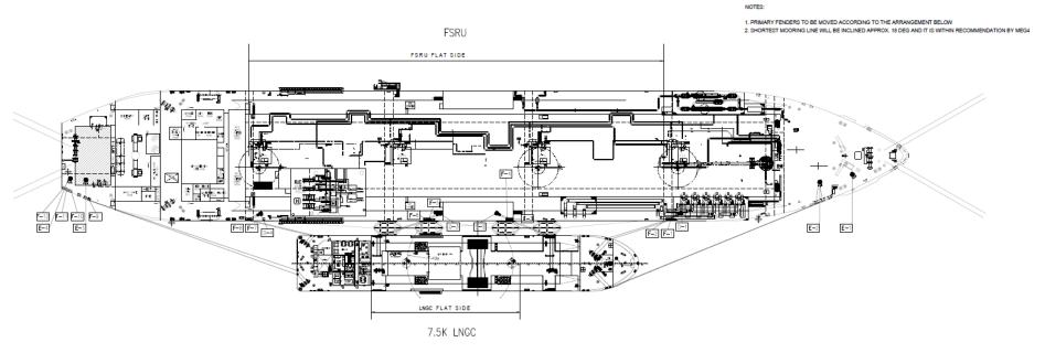
Figure 17 Proposed mooring plan with up to 7500 LNGC
