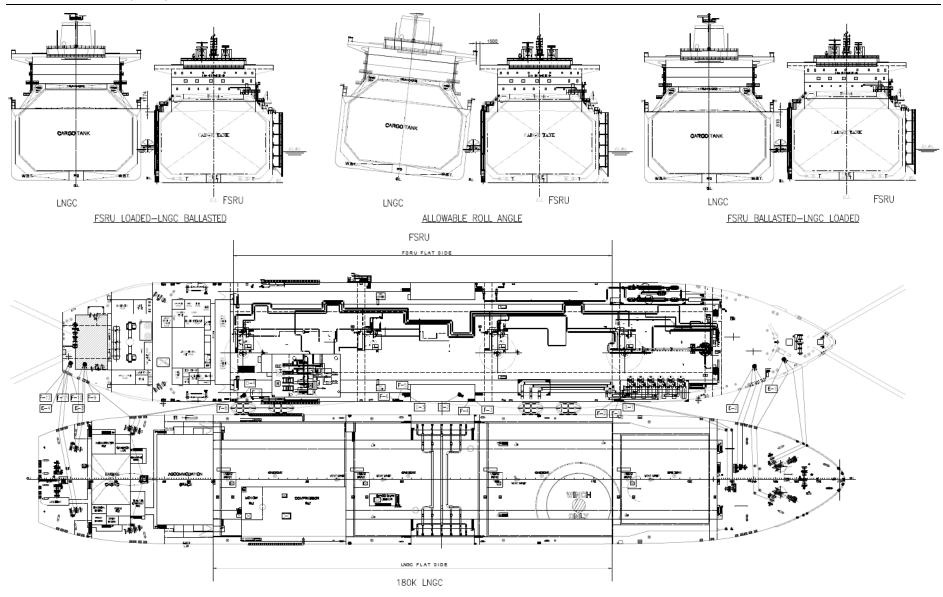
Figure 22 Proposed mooring plan with up to 180000 LNGC
