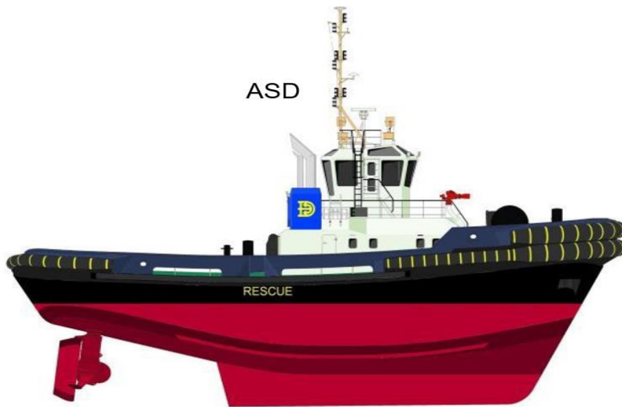
Figure 1: Azimuth Stern Drive.
