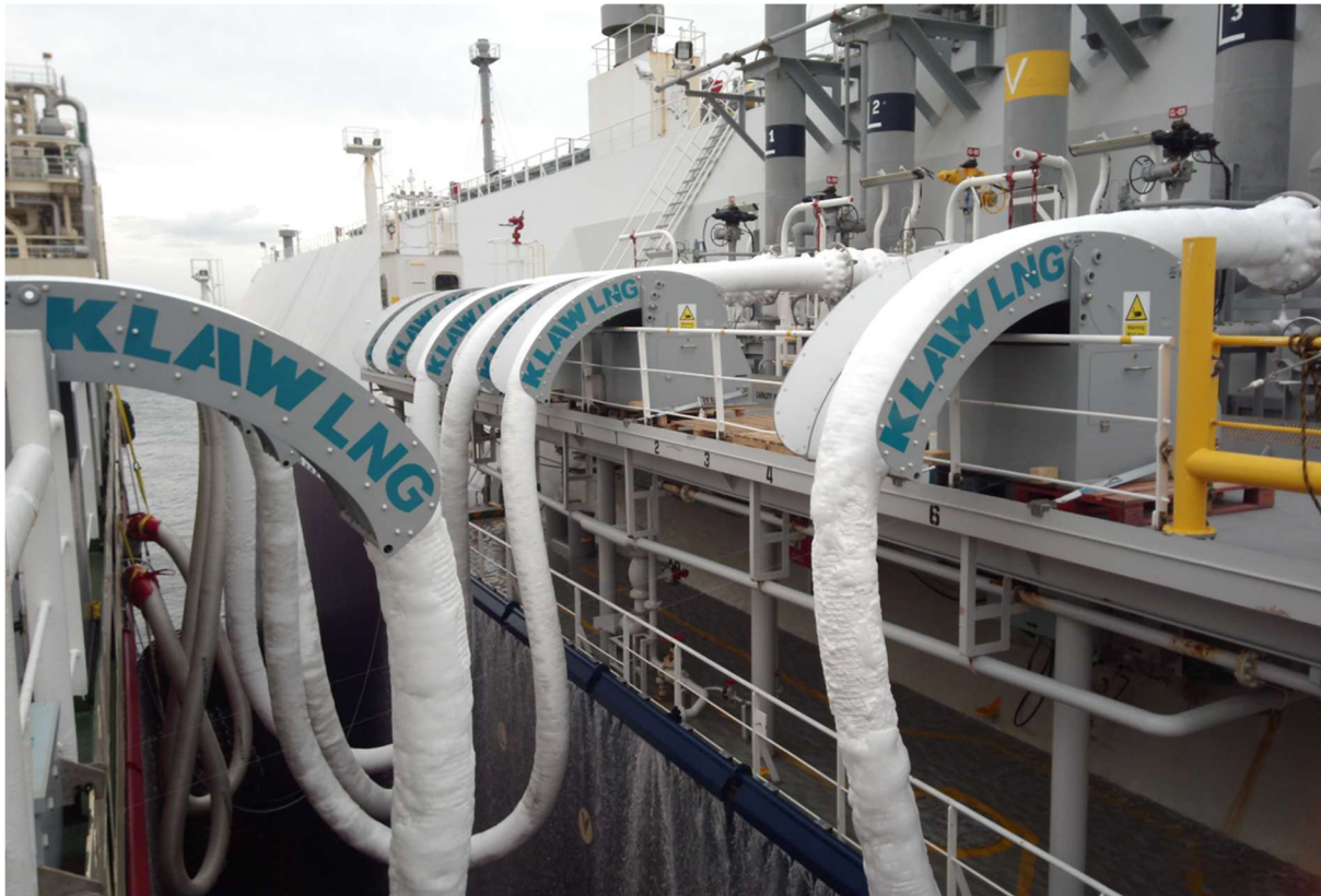
Figure 9 Flexible Hoses during Cargo Operation
