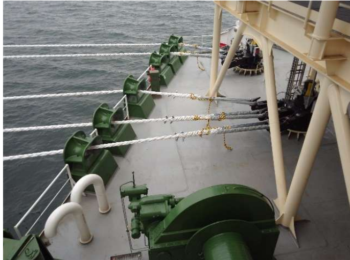
Figure 26 Stern Lines Mooring
