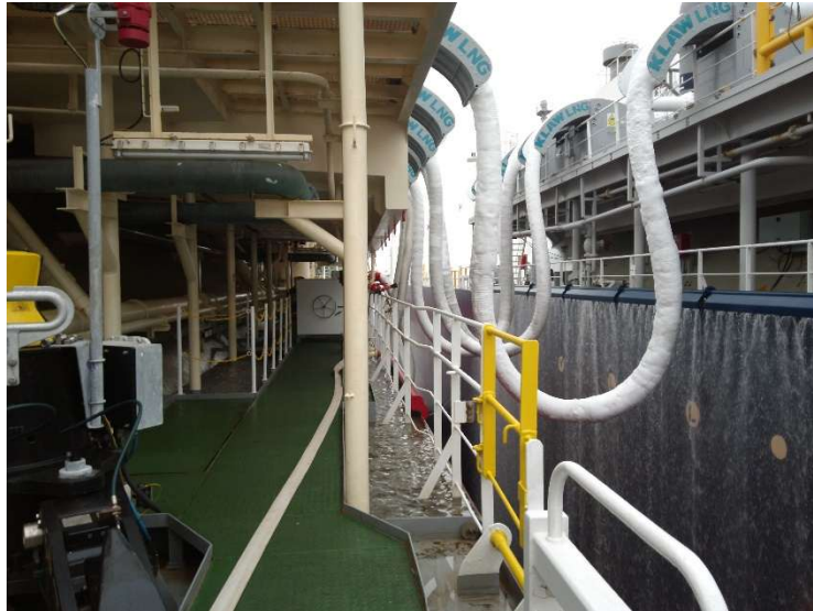
Figure 32 Water Curtain / Deluge
