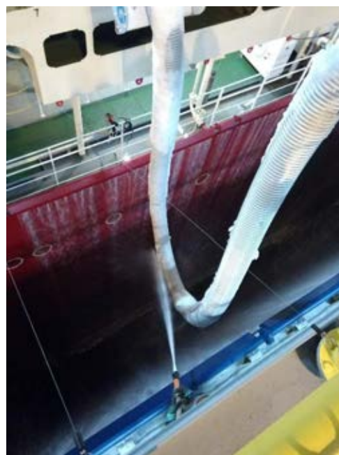
Figure 33 Hose Water spray process
