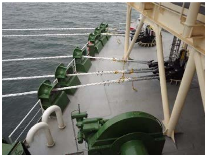
Figure 26 Stern Lines Mooring
